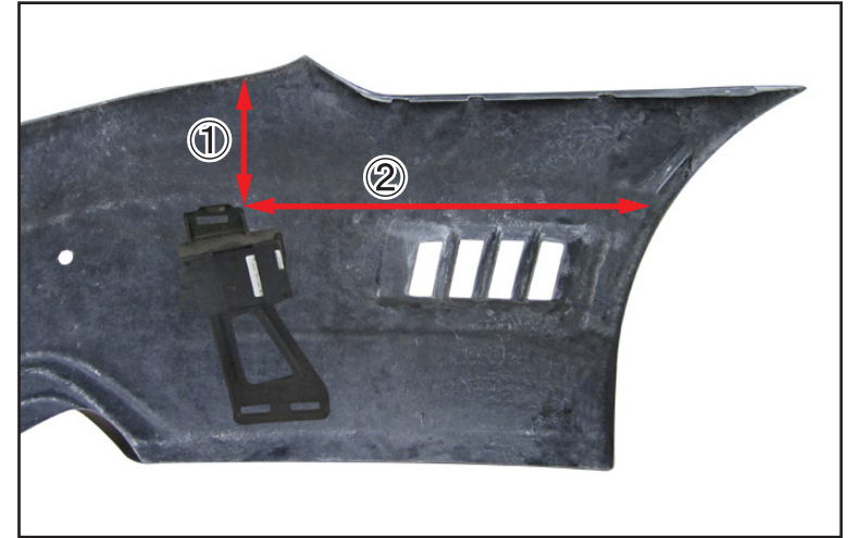
Use caulking glue to fix OEM brackets for PTS to WALD Rear Bumper. Location for PTS : Relocate OEM sensors and brackets as they were on OEM rear bumper.
