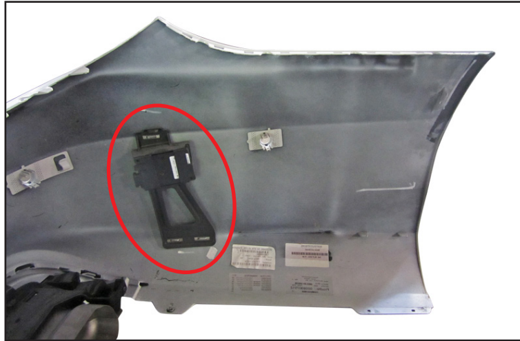
Replace the red circled OEM sensor and brackets to WALD Rear Bumper.
