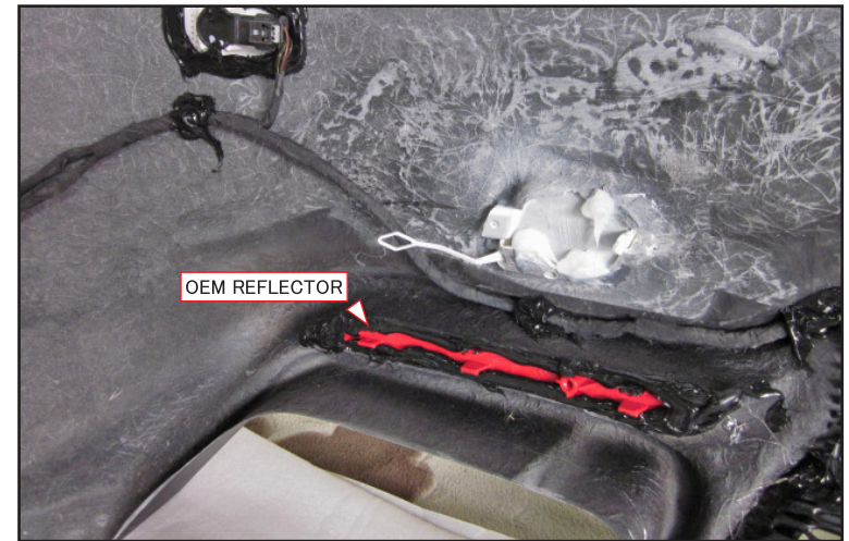
Use caulking glue to fix OEM reflectors from the rear on both right and left ducts.
